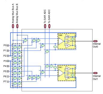
The ovals in Figure 4 represent analog switches, which may be controlled via user firmware, the SAR sequencer, or user-defined programmable logic. The opamps (OA0 and OA1) are configurable via these switches to perform all standard opamp functions with appropriate feedback components.
