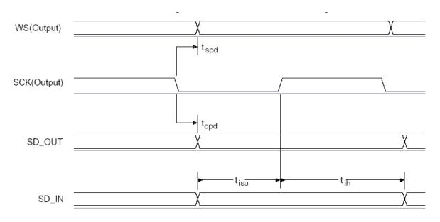
Figure 23: Digital audio interface master timing
