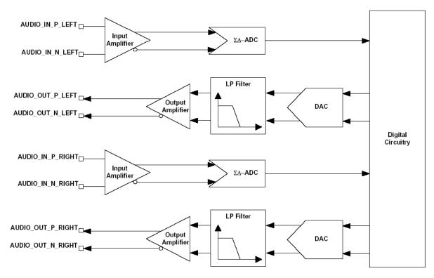
Figure 13: Stereo CODEC audio input and output stages
