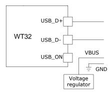
Figure 10: USB in bus powered mode
