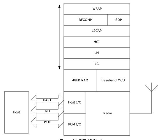
Figure 34: iWRAP Stack
