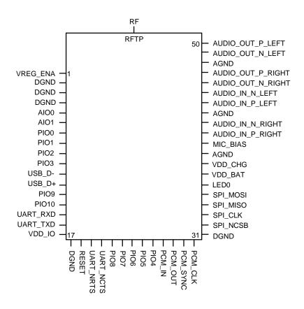
Figure 2: WT32 connection diagram (top view)
