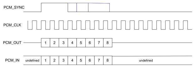
Figure 26: Long frame sync (shown with 8-bit companded sample)
