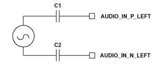
Figure 18: Differential input (left channel shown)
