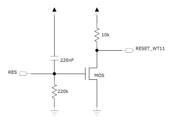
Figure 3: WT32 internal reset circuitry
