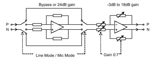
Microphone Mode input impedance =  $6k\Omega$ Line mode input impedance =  $6k\Omega$  to  $30k\Omega$
