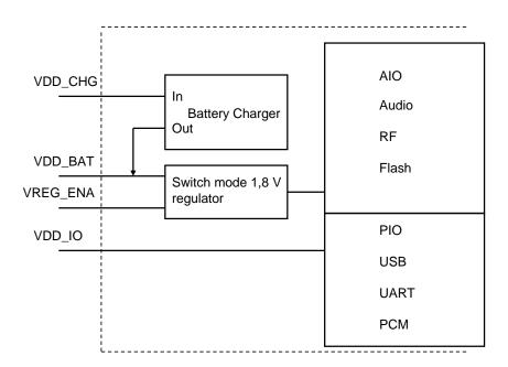
Figure 4: Power supply configuration of WT32
