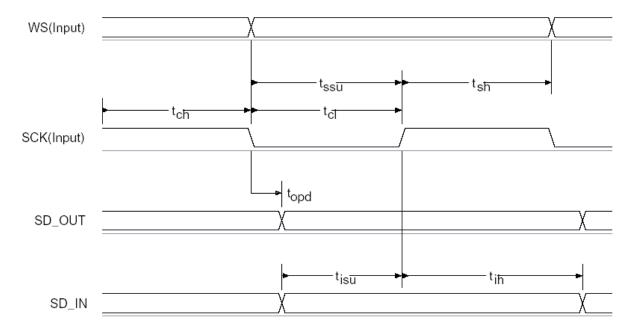
Figure 22: Digital audio interface slave timing
