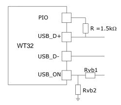
Figure 9: USB in self powered mode
