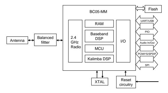
Figure 1: Block diagram of WT32
