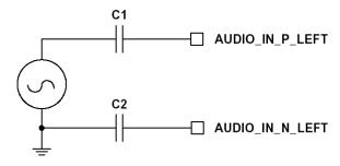
Figure 19: Single ended input (left channel shown)
