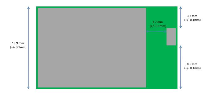
Figure 41: WT32 physical dimensions
