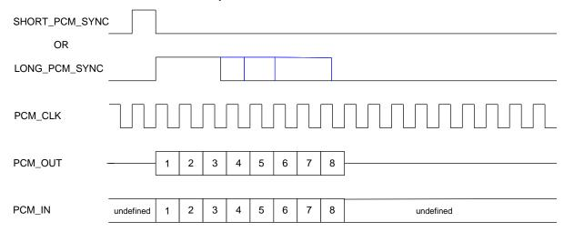
Figure 28: Multi slot operation with two slots and 8-bit companded samples
