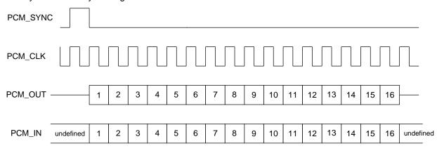
Figure 27: Short frame sync (shown with 16-bit companded sample)
