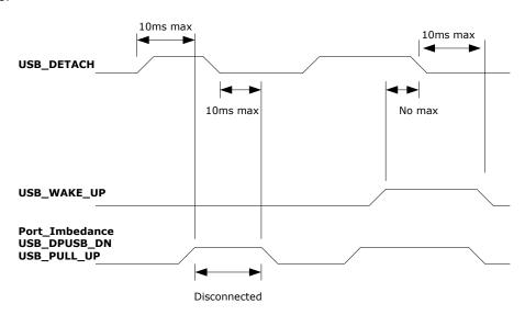
Figure 11: USB\_DETACH and USB\_WAKE\_UP Signal
