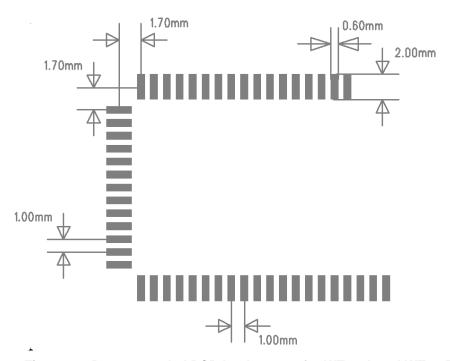
Figure 39: Recommended PCB land pattern for WT32-A and WT32-E
