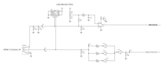
Figure 15: Example circuit for SPDIF interface (Co-Axial)
