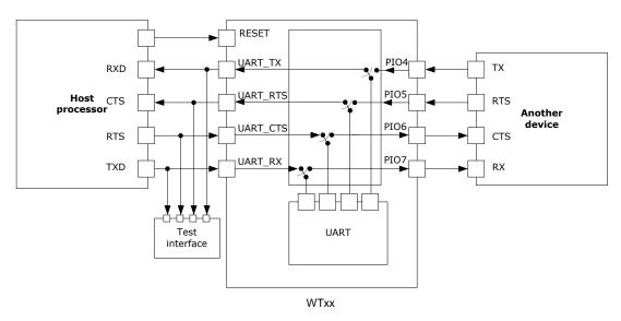
Figure 8: UART bypass mode
