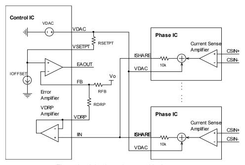
Figure 8 - Adaptive voltage positioning
