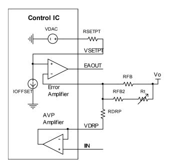
Figure 9 - Temperature compensation of inductor DCR
