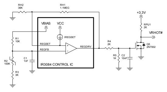
Figure 12b – IR3084A Bias Regulator configured for VRHOT# Function
