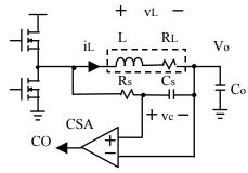
Figure 6 - Inductor Current Sensing and Current Sense Amplifier
