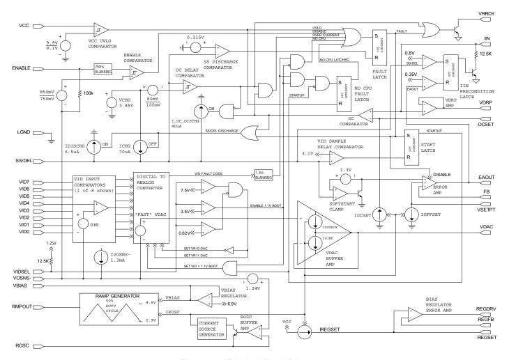
Figure 7 – IR3084A Block Diagram
