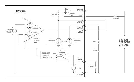
Figure 1 – System Set Point Test Circuit
