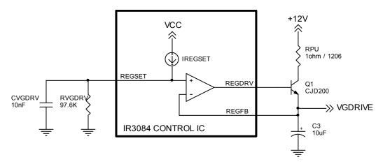
Figure 12a – IR3084A Bias Regulator configured for Gate Driver Bias Regulator
