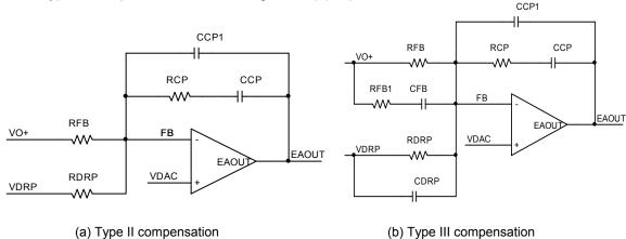
Figure 20: Voltage Loop Compensation Networks
