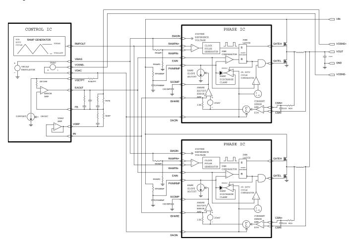
Figure 3 - IR3084A PWM Block Diagram
