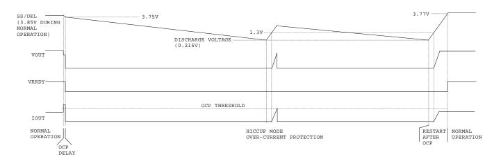
Figure 11 – Over-Current Protection Waveforms (VID = 1.1V for simplicity)
