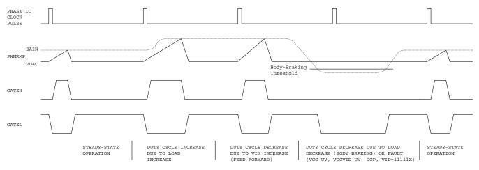
Figure 5 - PWM Operating Waveforms
