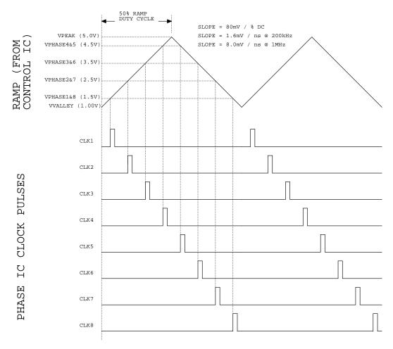
Figure 4 – 8 Phase Oscillator Waveforms
