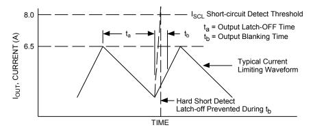
Figure 9. Active Current Limiting Detail
