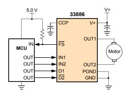
Figure 1. 33886 Simplified Application Diagram
