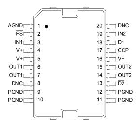
Figure 3. 33886 Pin Connections
