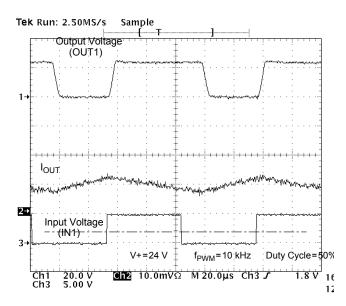
Figure 14. Output Voltage and Current vs. Input Voltage at V+ = 24 V, PMW Frequency of 10 kHz, and Duty Cycle of 50%
