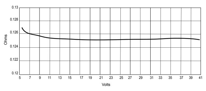
Figure 19. Typical Low Side  $R_{DS(ON)}$  Versus V+
