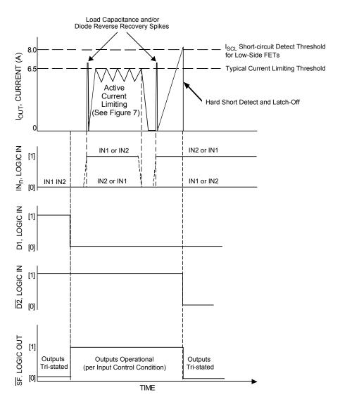
Figure 8. Active Current Limiting Versus Time
