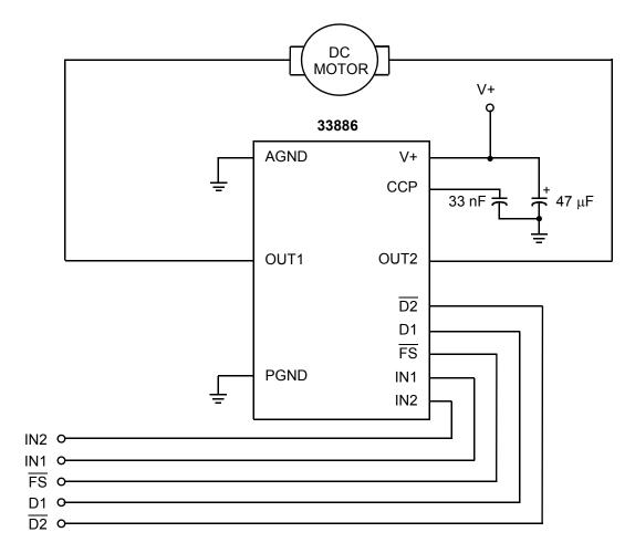
Figure 23. 33886 Typical Application Schematic
