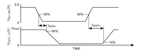
Figure 4. Output Delay Time
