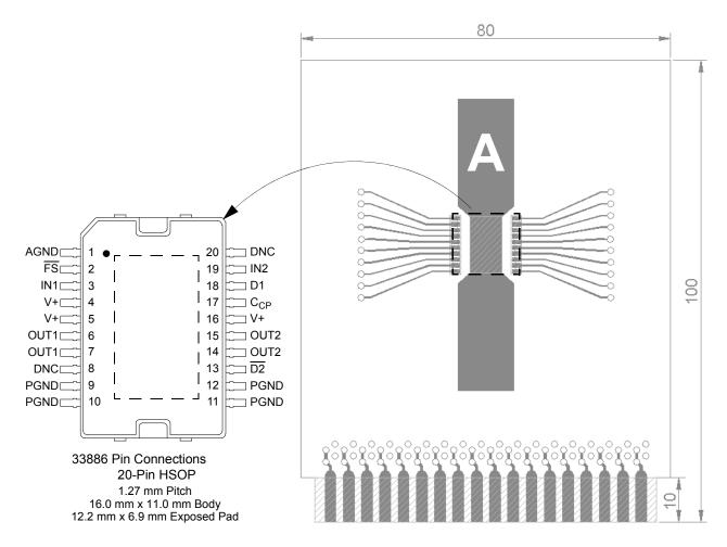
Figure 25. Thermal Test Board
