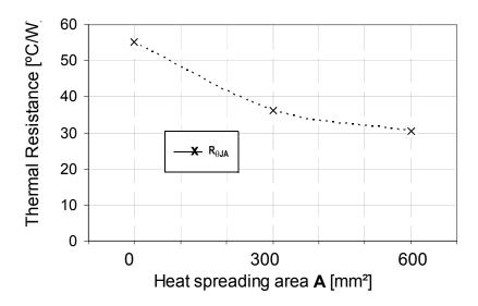
Figure 26. Device on Thermal Test Board  $\textbf{R}_{\theta \text{JA}}$
