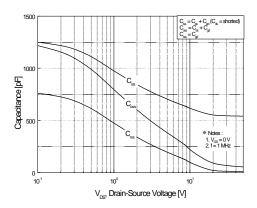
Figure 5. Capacitance Characteristics
