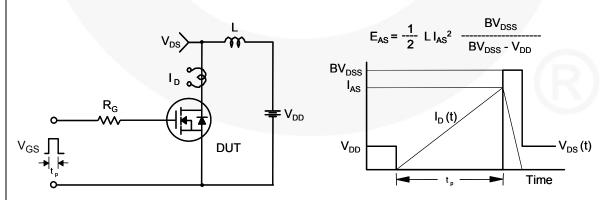
Figure 14. Unclamped Inductive Switching Test Circuit & Waveforms
