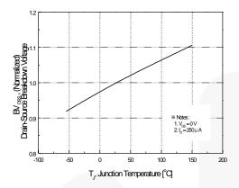
Figure 7. Breakdown Voltage Variation vs. Temperature
