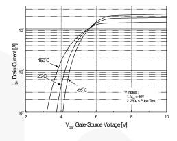
Figure 2. Transfer Characteristics
