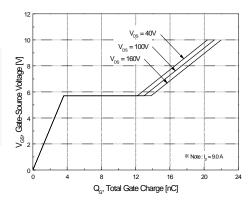
**Figure 6. Gate Charge Characteristics**
