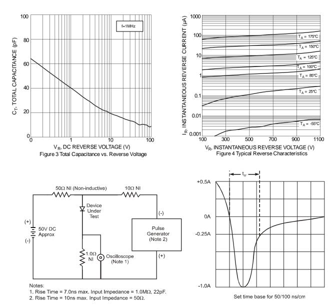
Figure 5 Reverse Recovery Time Characteristic and Test Circuit
