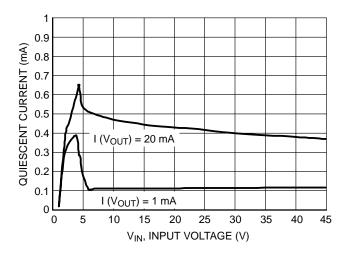
Figure 3. Quiescent Current vs. Input Voltage (Operating Mode)
