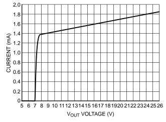
Figure 15. V<sub>OUT</sub> Short to Battery
