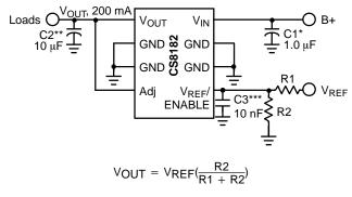
Figure 9. Tracking Regulator at Lower Voltages
