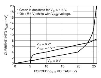
Figure 5. V<sub>OUT</sub> Reverse Current
