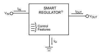
Figure 17. Single Output Regulator with Key Performance Parameters Labeled
