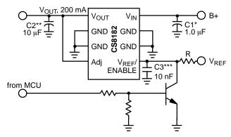
Figure 10. Tracking Regulator with ENABLE Circuit
