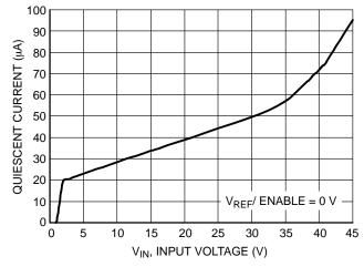
Figure 4. Quiescent Current vs. Input Voltage (Sleep Mode)
