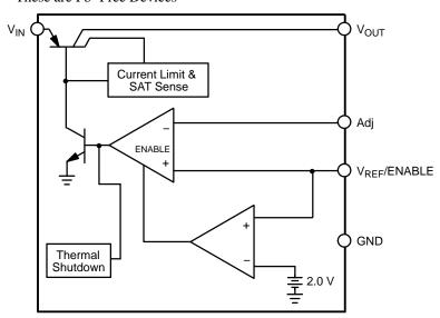
Figure 1. Block Diagram
