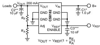
Figure 8. Tracking Regulator at Higher Voltages
