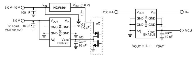
Figure 11. Alternative ENABLE Circuit
