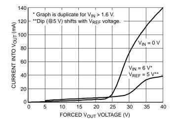
Figure 6. V<sub>OUT</sub> Reverse Current
