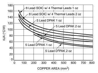
Figure 20. 5 Lead D<sup>2</sup>PAK Thermal Resistance
