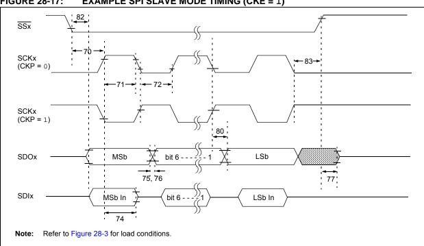
FIGURE 28-17: **EXAMPLE SPI SLAVE MODE TIMING (CKE = 1)**
