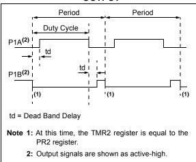
FIGURE 19-5: EXAMPLES OF HALF-BRIDGE OUTPUT MODE APPLICATIONS
