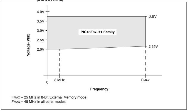
FIGURE 28-2: PIC18F87J11 FAMILY VOLTAGE-FREQUENCY GRAPH, REGULATOR DISABLED (INDUSTRIAL)()
