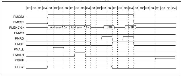
FIGURE 12-26: WRITE TIMING, 16-BIT MULTIPLEXED DATA, FULLY MULTIPLEXED 16-BIT ADDRESS
