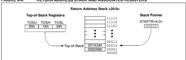
FIGURE 6-4: RETURN ADDRESS STACK AND ASSOCIATED REGISTERS
