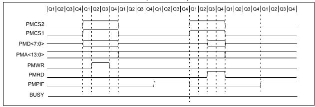
FIGURE 12-13: READ TIMING, 8-BIT DATA, PARTIALLY MULTIPLEXED ADDRESS
