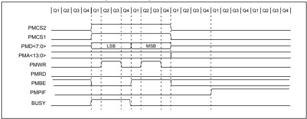
FIGURE 12-23: READ TIMING, 16-BIT MULTIPLEXED DATA, PARTIALLY MULTIPLEXED ADDRESS
