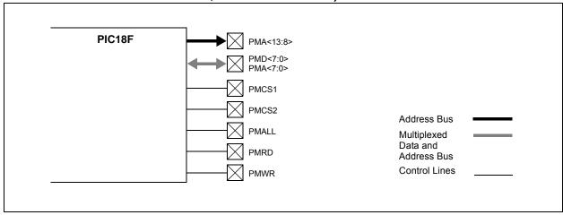
FIGURE 12-11: FULLY MULTIPLEXED ADDRESSING MODE (SEPARATE READ AND WRITE STROBES, TWO CHIP SELECTS)
