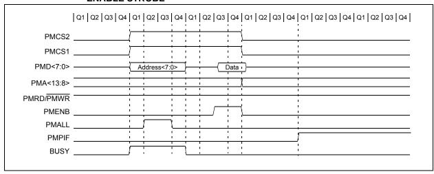
FIGURE 12-18: WRITE TIMING, 8-BIT DATA, PARTIALLY MULTIPLEXED ADDRESS, ENABLE STROBE
