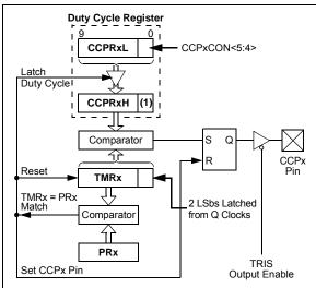
Note 1: The two LSbs of the Duty Cycle register are held by a 2-bit latch that is part of the module's hardware. It is physically separate from the CCPRx registers.
