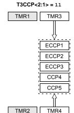
Timer3 is used for all Capture and Compare operations for all CCP modules. Timer4 is used for PWM operations for all CCP modules. Modules may share either timer resource as a common time base.
