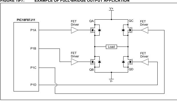
**FIGURE 19-7: EXAMPLE OF FULL-BRIDGE OUTPUT APPLICATION**
