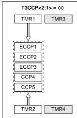
Timer1 is used for all Capture and Compare operations for all CCP modules. Timer2 is used for PWM operations for all CCP modules. Modules may share either timer resource as a common time base.
