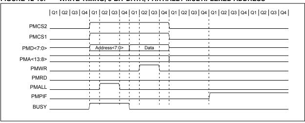
FIGURE 12-16: WRITE TIMING, 8-BIT DATA, WAIT STATES ENABLED, PARTIALLY MULTIPLEXED ADDRESS
