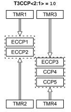
Timer1 and Timer2 are used for Capture and Compare or PWM operations for ECCP1 and ECCP2 only (depending on the mode selected for each module). Both modules may use a timer as a common time base if they are both in Capture/Compare or PWM modes.
