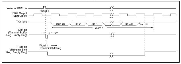
FIGURE 21-5: ASYNCHRONOUS TRANSMISSION (BACK-TO-BACK)
