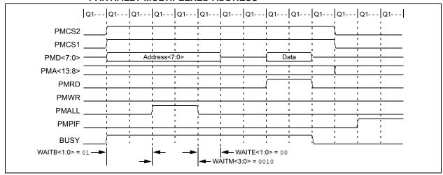
FIGURE 12-15: WRITE TIMING, 8-BIT DATA, PARTIALLY MULTIPLEXED ADDRESS
