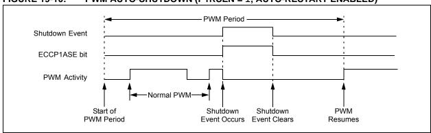
FIGURE 19-10: PWM AUTO-SHUTDOWN (P1RSEN = 1, AUTO-RESTART ENABLED)
