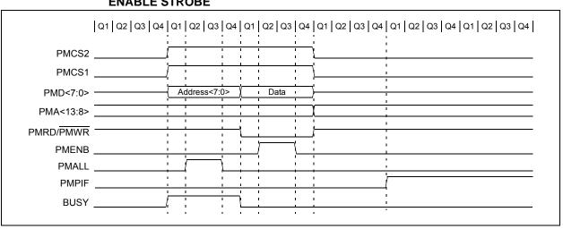
FIGURE 12-19: READ TIMING, 8-BIT DATA, FULLY MULTIPLEXED 16-BIT ADDRESS
