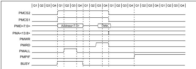
FIGURE 12-14: READ TIMING, 8-BIT DATA, WAIT STATES ENABLED, PARTIALLY MULTIPLEXED ADDRESS
