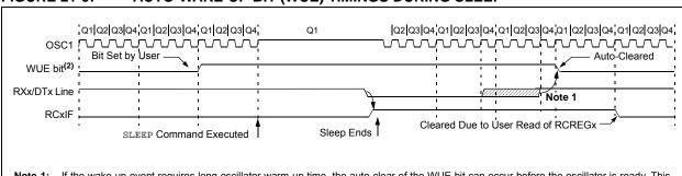
Note 1: If the wake-up event requires long oscillator warm-up time, the auto-clear of the WUE bit can occur before the oscillator is ready. This sequence should not depend on the presence of Q clocks.
