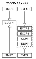
Timer1 and Timer2 are used for Capture and Compare or PWM operations for ECCP1 only (depending on selected mode).
