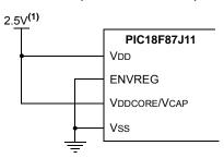
Note 1: These are typical operating voltages. Refer to Section 28.1 "DC Characteristics: Supply Voltage" for the full operating ranges of VDD and VDDCORE.
