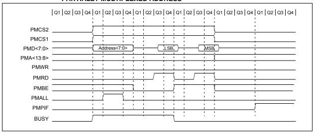
FIGURE 12-24: WRITE TIMING, 16-BIT MULTIPLEXED DATA, PARTIALLY MULTIPLEXED ADDRESS
