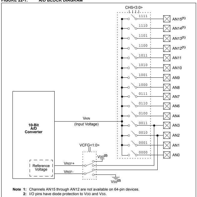
After the A/D module has been configured as desired, the selected channel must be acquired before the conversion is started. The analog input channels must have their corresponding TRIS bits selected as an input. To determine acquisition time, see **Section 22.1** "A/D Acquisition Requirements". After this acquisition time has elapsed, the A/D conversion can be started. An acquisition time can be programmed to occur between setting the GO/DONE bit and the actual start of the conversion.
