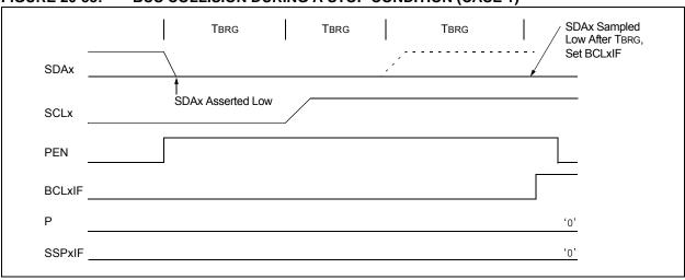
FIGURE 20-34: BUS COLLISION DURING A STOP CONDITION (CASE 2)
