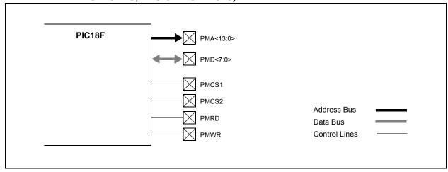
FIGURE 12-10: PARTIALLY MULTIPLEXED ADDRESSING MODE (SEPARATE READ AND WRITE STROBES, TWO CHIP SELECTS)
