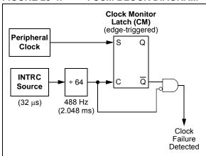
Clock failure is tested for on the falling edge of the sample clock. If a sample clock falling edge occurs while CM is still set, a clock failure has been detected (Figure 25-5). This causes the following:
