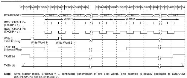
FIGURE 21-12: SYNCHRONOUS TRANSMISSION (THROUGH TXEN)
