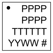
Figure 9.3. QFN20 Package Marking
