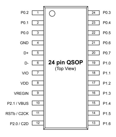
Figure 6.1. EFM8UB3x-QSOP24 Pinout
