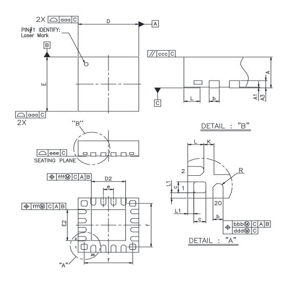
Figure 9.1. QFN20 Package Drawing
