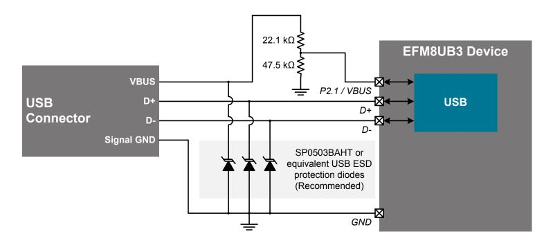
Figure 5.5. Self-Powered Connection Diagram for USB Pins
