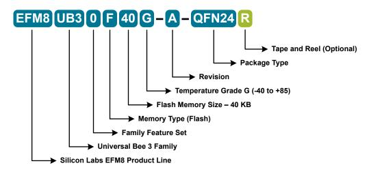
Figure 2.1. EFM8UB3 Part Numbering
