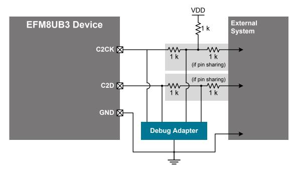
Figure 5.6. Debug Connection Diagram
