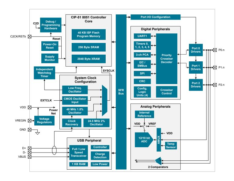
Figure 3.1. Detailed EFM8UB3 Block Diagram
