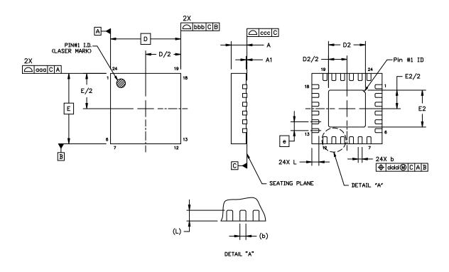
Figure 7.1. QFN24 Package Drawing
