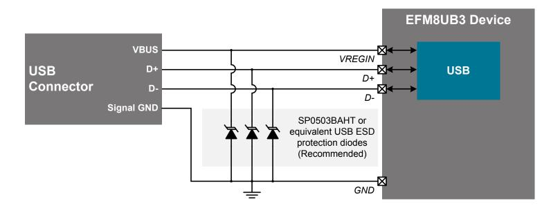
Figure 5.4. Bus-Powered Connection Diagram for USB Pins
