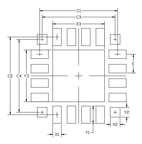
Figure 9.2. QFN20 PCB Land Pattern Drawing
