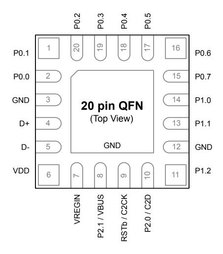
Figure 6.3. EFM8UB3x-QFN20 Pinout
