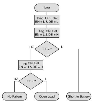
Figure 20. Flowchart for Diagnostics in OFF State
