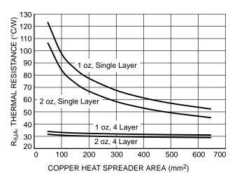
Figure 22. Thermal Resistance vs. PCB Copper Area
