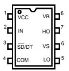
Figure 4. Pin Assignment (Top Through View)
