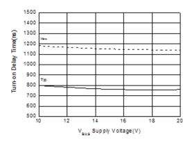
Figure 16. Turn-on Delay Time of HO vs. V<sub>BS</sub> Supply Voltage (V<sub>CC</sub>=15 V, C<sub>L</sub>=1 nF, T<sub>A</sub>=25°C)
