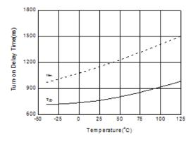
Figure 15. Turn-on Delay Time of HO vs. Temperature ( $V_{CC}=V_{BS}=15 V$ ,  $C_{L}=1 nF$ )
