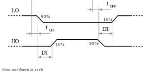
Figure 14. **Dead Time Waveform Definitions**
