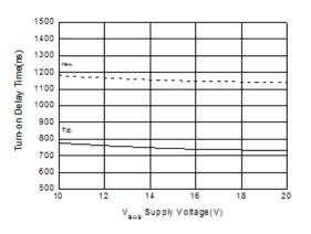
Figure 18. Turn-on Delay Time of LO vs. V<sub>BS</sub> Supply Voltage (V<sub>CC</sub>=15 V, C<sub>L</sub>=1 nF, T<sub>A</sub>=25°C)
