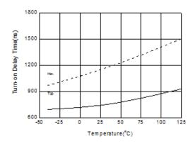
Figure 17. Turn-on Delay Time of LO vs. Temperature ( $V_{CC}=V_{BS}=15 V$ ,  $C_L=1 nF$ )
