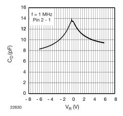
Fig. 3 - Typical Capacitance C<sub>D</sub> vs. Reverse Voltage V<sub>R</sub>
