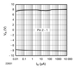
Fig. 4 - Typical Reverse Voltage V<sub>R</sub> vs. Reverse Current I<sub>R</sub>
