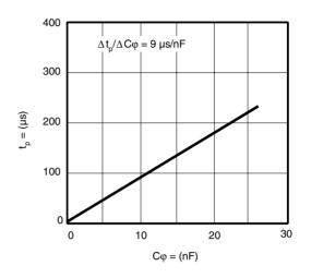
Figure 8. Soft-start Charge Current
