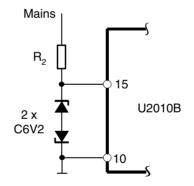
If the mains voltage compensation and the automatic retriggering are not required, both functions can be suppressed by limiting  $|V_{15-10}| \le 7 \text{ V}$ , see Figure 4.
