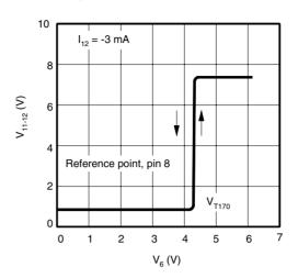
Figure 14. Overload Switching
