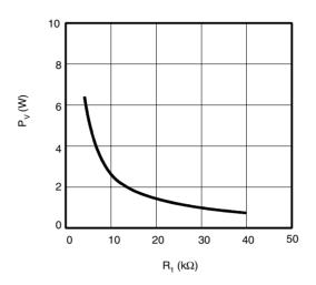
Figure 17. Power Dissipation of R<sub>1</sub> According to Current Consumption
