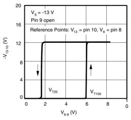
Figure 13. High Load Switching (70%)
