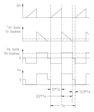
Figure 2: Discontinuous Mode Flyback Waveforms
