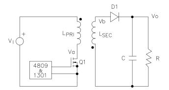
Figure 1: Flyback Power Converter
