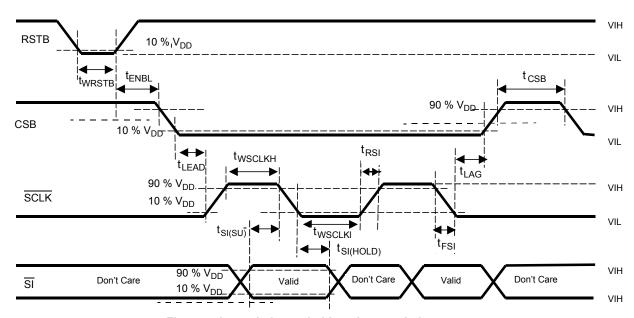
Figure 7. Input timing switching characteristics
