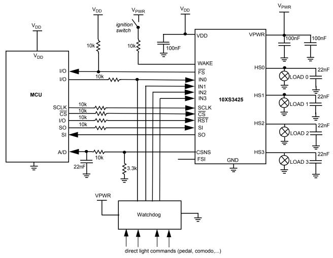
Figure 16. Typical automotive lighting (one corner)
