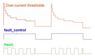
In steady state, the wire harness will be protected by a OCLO2 current level by default. Three other DC overcurrent levels are available: OCLO1, or OCLO3, or OCLO4, based on the state of the OCLO[1,0] bits.
