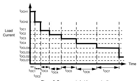
Figure 5. Overcurrent shutdown protection
