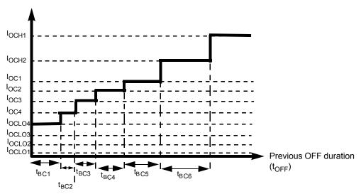
Figure 6. Bulb cooling management
