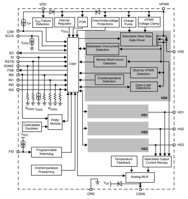
Figure 2. 10XS3425 simplified internal block diagram
