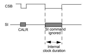
In case a negative CSB pulse is outside a predefined time range (from  $t_{CSB(MIN)}$  to  $t_{CSB(MAX)}$ ), the calibration event will be ignored and the internal clock will be unaltered, or reset to the default value ( $f_{PWM(0)}$ ), if this was not calibrated before.
