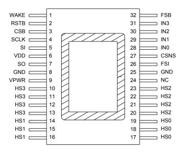
Figure 3. 10XS3425 pin connections
