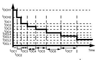
Figure 14. Overcurrent profile depending on xenon bit
