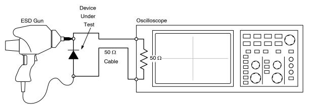
Figure 4. Diagram of ESD Test Setup
