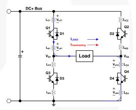
Figure 36. Q1 and Q4 Turn-On
