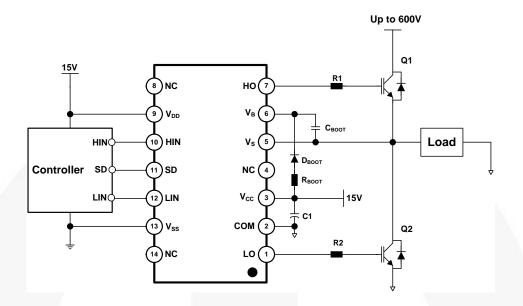
Figure 1. Typical Application Circuit (Referenced 14-DIP)
