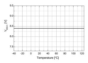
Figure 20. V<sub>BS</sub> UVLO+ vs. Temperature
