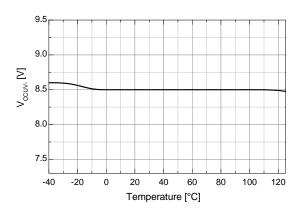
Figure 18. V<sub>CC</sub> UVLO+ vs. Temperature
