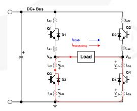
Figure 37. Q1 Turn-Off and D3 Conducting
