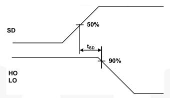
Figure 32. Shutdown Waveform Definition
