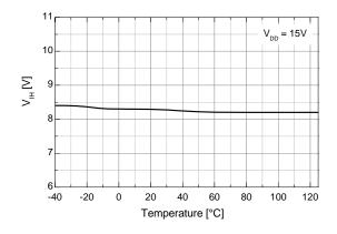
Figure 24. Logic High Input Voltage vs. Temperature
