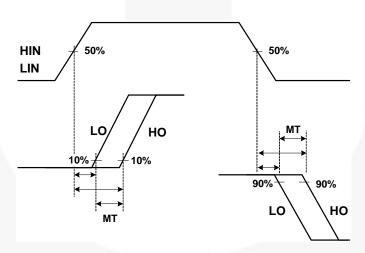
Figure 33. Delay Matching Waveform Definitions
