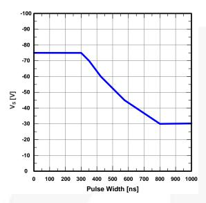
Figure 38. Negative V<sub>S</sub> Transient Chracteristic
