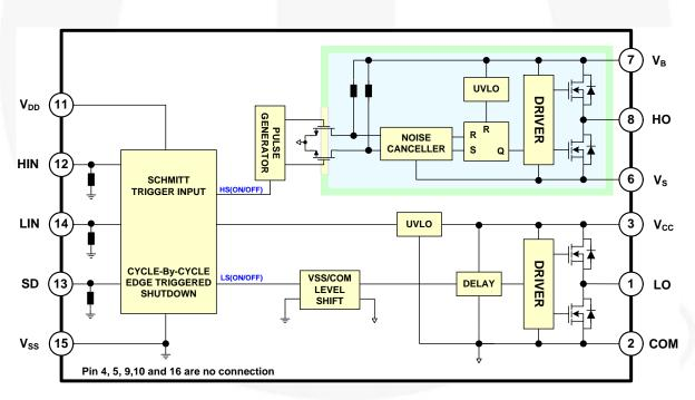
Figure 4. Functional Block Diagram (Referenced 16-SOP)
