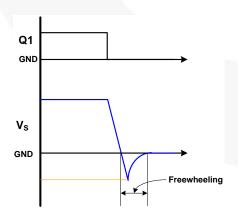
Figure 35. V<sub>S</sub> Waveforms During Q1 Turn-Off
