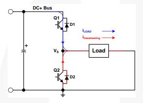
Figure 34. Half-Bridge Application Circuits
