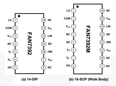
Figure 5. Pin Configurations (Top View)
