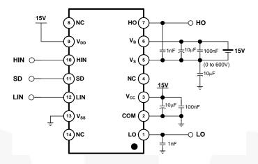
Figure 29. Switching Time Test Circuit (Referenced 14-DIP)
