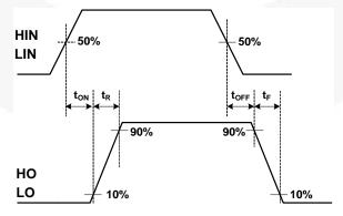
Figure 31. Switching Time Waveform Definitions
