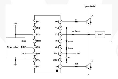
Figure 2. Typical Application Circuit (Referenced 16-SOP)
