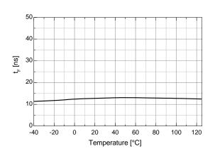
Figure 8. Turn-On Rise Time vs. Temperature
