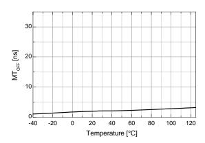
Figure 10. Turn-On Delay Matching vs. Temperature
