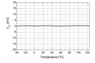
Figure 22. High-Level Output Voltage vs. Temperature
