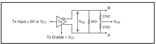
FIGURE 8. RS-485/422 DRIVER OUTPUT SHORT CIRCUIT CURRENT
