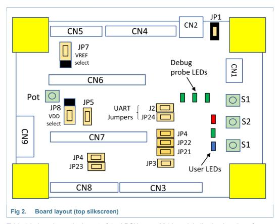
Table 1 below shows the layout of the LPCXpresso804 board, indicating location of jumpers, buttons, connectors/expansion options and MCU devices.
