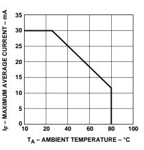
Figure 3. Maximum Allowable Average Current per Dot vs. Ambient Temperature.
