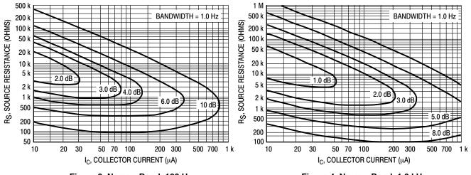
Figure 3. Narrow Band, 100 Hz
