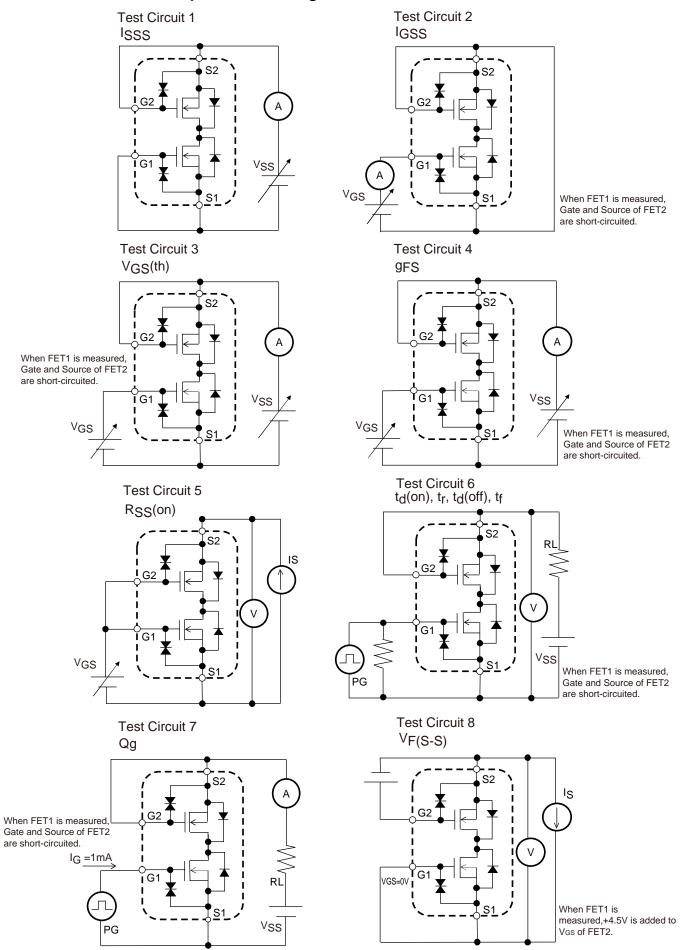
When FET2 is measured, the position of FET1 and FET2 is switched.
