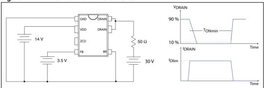
Figure 5. Brown-out threshold test circuits
