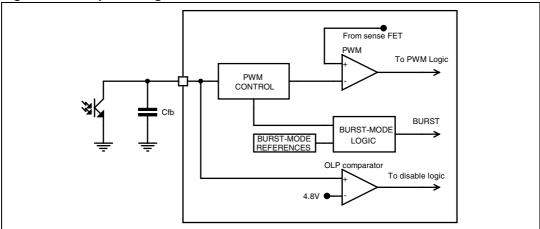
Figure 35. FB pin configuration
