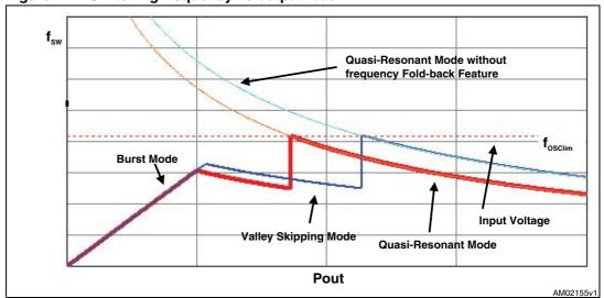
Figure 27. Switching frequency vs output load
