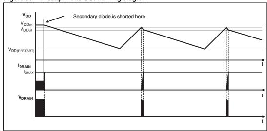
Figure 39. Hiccup-mode OCP: timing diagram
