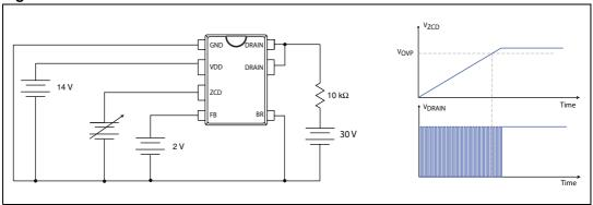
Note: Adjust  $V_{DD}$  above  $V_{DDon}$  start-up threshold before settings to 14 V
