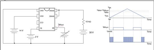
Figure 6. OVP threshold test circuits
