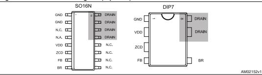
Note: The copper area for heat dissipation has to be designed under the DRAIN pins.
