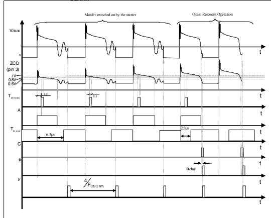
Figure 30. Double T<sub>BLANK</sub> timing diagram
