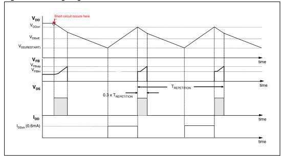
Figure 26. Timing diagram: behavior after short circuit
