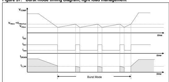
Figure 37. Burst mode timing diagram, light load management
