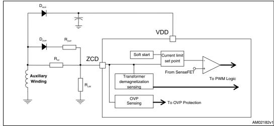
Figure 32. ZCD pin typical external configuration
