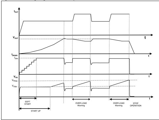
Figure 36. Timing diagram: Overload protection
