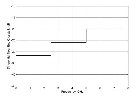
Figure 3: Illustration of different ial near end crosstalk requirement.
