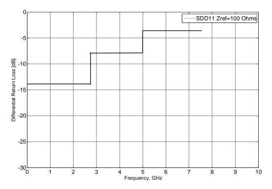
Figure 2: Illustration of differential return loss requirement.
