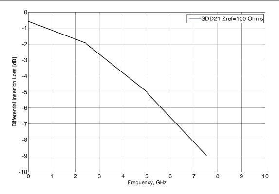
Figure 1: Illustration of differential insertion loss requirement.
