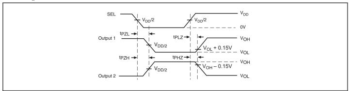
**Voltage Waveforms Enable and Disable Times**
