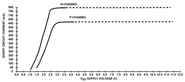
FIGURE 7. TYPICAL CHARACTERISTIC OF THE P AND N OUTPUT DRIVER SHORT CIRCUIT CURRENT vs SUPPLY VOLTAGE, T<sub>AMBIENT</sub> =  $25^{\circ}$ C
