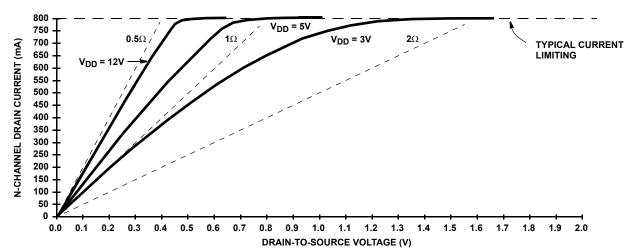
FIGURE 6. TYPICAL CHARACTERISTIC OF THE N-MOSFET OUTPUT DRIVER DRAIN CURRENT vs DRAIN-TO-SOURCE VOLTAGE, T<sub>AMBIENT</sub> = 25°C
