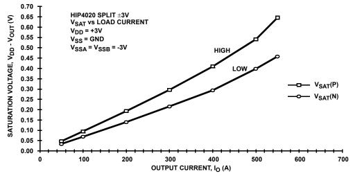
FIGURE 9. TYPICAL CHARACTERISTIC OF SATURATION VOLTAGE vs OUTPUT CURRENT USING A ±3V SPLIT SUPPLY, OUTPUT REFERENCE EQUAL LOGIC GROUND, T<sub>AMBIENT</sub> = 25°C
