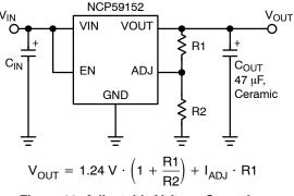
Figure 23. Adjustable Voltage Operation
