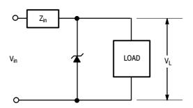
**Figure 3. Typical Protection Circuit**
