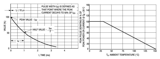
Figure 1. 10  $\times$  1000  $\mu s$  Pulse Waveform
