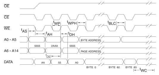
1. A6 through A14 must specify the same page address during each high to low transition of WE (or CE) after the software Notes: code has been entered.
