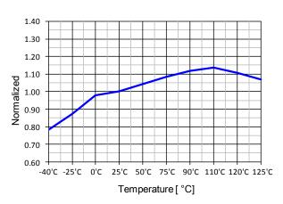
Figure 6. Startup Charging Current (I<sub>CH</sub>) vs. T<sub>A.</sub>
