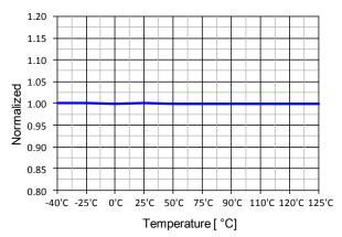
Figure 14. Switching Frequency (fs) vs. TA.
