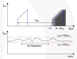
Figure 26. Random Frequency Fluctuation
