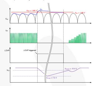
Figure 24. Line Over-Voltage Protection
