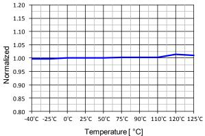
Figure 10. UVLO Threshold Voltage (V<sub>START</sub>) vs. T<sub>A</sub>.
