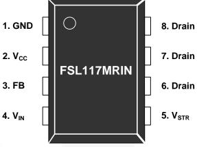
Figure 3. Pin Assignments (Top View)
