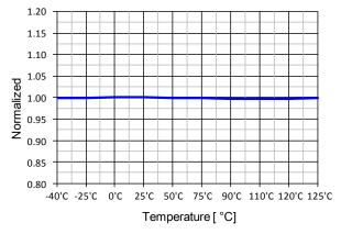
Figure 12. Shutdown Feedback Voltage (V<sub>SD</sub>) vs. T<sub>A.</sub>
