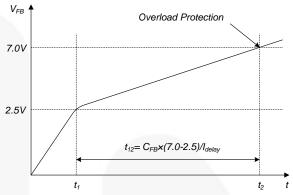
Figure 21. Overload Protection
