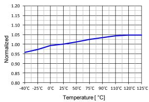
Figure 8. Feedback Source Current (IFB) vs. TA.
