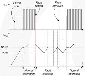
Figure 20. Auto-Restart Protection Waveforms
