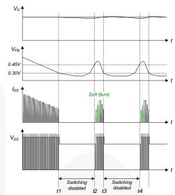
Figure 25. Burst-Mode Operation
