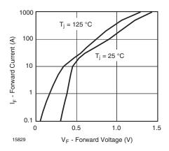
Fig. 3 - Forward Current vs. Forward Voltage
