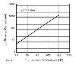
Fig. 2 - Reverse Current vs. Junction Temperature
